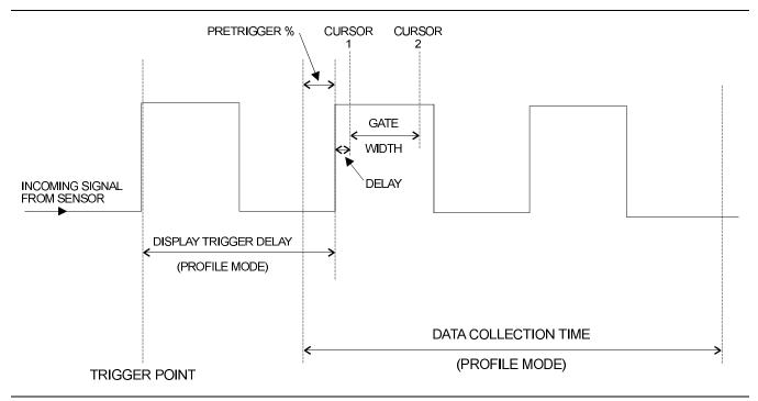
Figure 4-4. Sample Trigger in Graphic Mode
