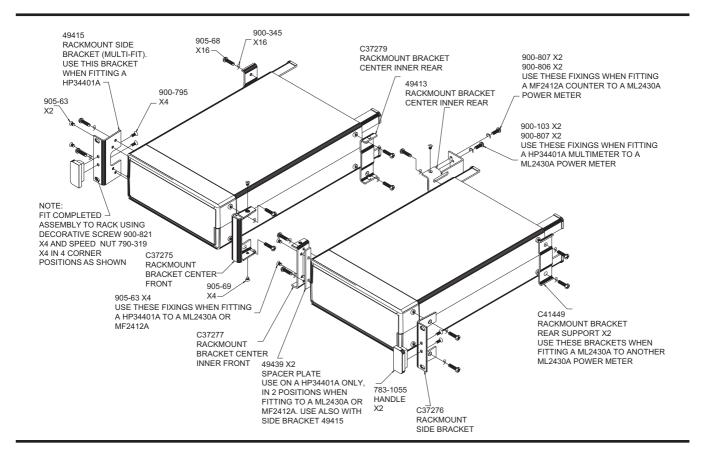
The procedure for fitting a ML2400A to a HP34401A Multimeter is as follows:
