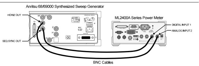
Figure 4-5. Source Sweep Mode Interconnection Example
