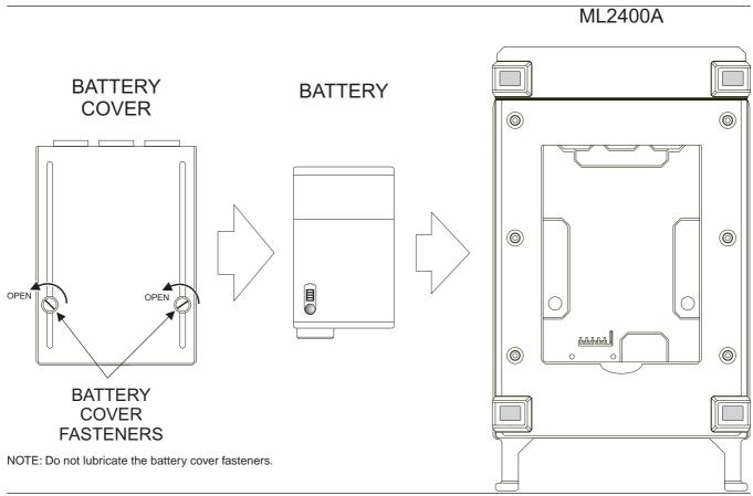
Figure 2-1. Model ML2400A Series Battery Compartment
