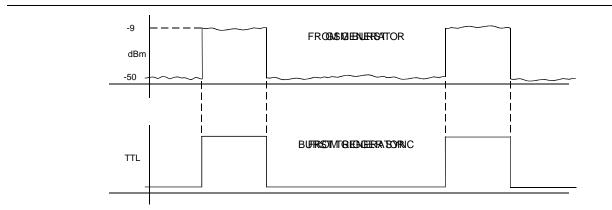
Figure 4-3. Typical Arming Diagram
